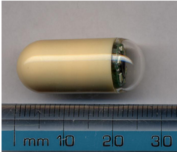
Figure 1. Video capsule endoscopy, also known as Pillcam ® , is an easy to swallow camera that navigates through the bowel and is excreted in the feces. 'Capsule endoscope' by Euchiasmus is licensed under CC BY 2.0. 5
